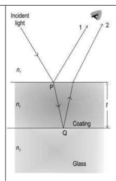
Reflected light undergoes a 180° phase shift when it falls on a denser medium from a rarer medium and no phase shift when it falls on a rarer medium from a denser medium. (Note: The thickness of coating is much less than the glass.) To answer the questions below, consider a monochromatic light of wavelength  $\lambda$  incident on the coating of thickness t at a small angle of incidence and n1<n2<n3. Also Consider PQ  $\approx$  t.
